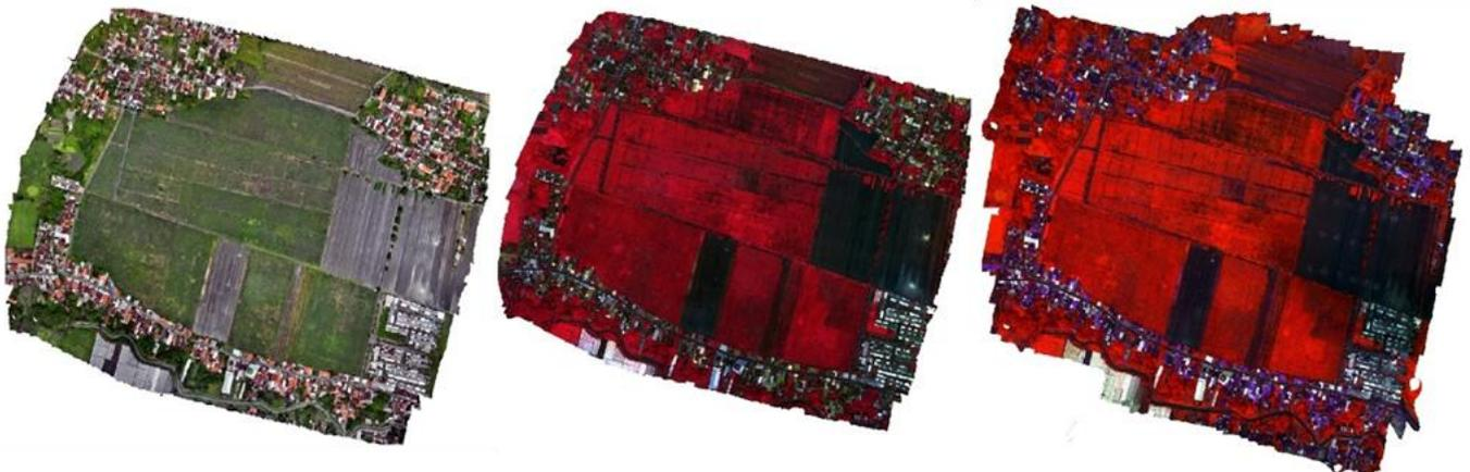
**Figure 4.** Orthophoto on multispectral camera compared to RGB Photo (left) DJI RGB Camera Color Aerial Photo; (Middle) Color Infrared Aerial Photo of DJI Mavic 3M Multispectral Camera and (right) Color Infrared Aerial Photo of MAPIR RGN Camera.
