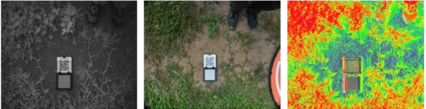
**Figure 3.** Micasense Calibrated Reflectance Panel (CRP) RP06-2123093-OB
